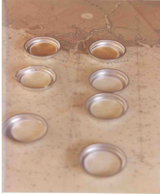
Figure 5: GF/F filters after filtration of water samples on Sofala bank, Mozambique. The filters have been laid on a chart to show their sampling location. Photo: D.G. Bowers.
