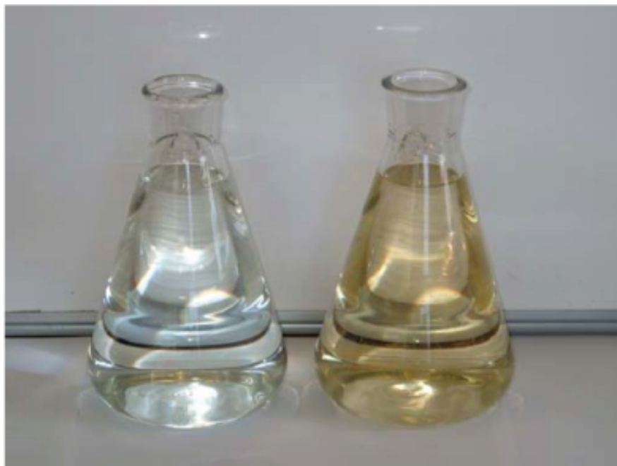
Figure 3: A flask of clear water (left) and one containing CDOM (right). Flask on the right was prepared by filtering coastal water through 0.2\mu m filters to remove particles. The coloration produced by CDOM in shelf seas and estuaries is sufficient to remotely sense its concentration using satellite ocean colour data. Photo: B. D. Moate
